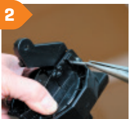
Using pliers remove the pivot pin.
