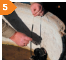
Apply anti-tangle tubing to the cord.
