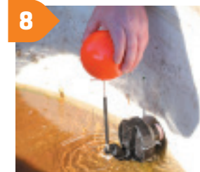
Water level can be adjusted by adjusting the length of cord at the float end. When desired level is set trim excess cord.
